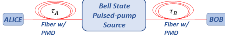
Figure 3.1: Schematic of the scenario of interest. A pulsed-pump source generates polarization-entangled photon pairs. The two photons of each pair are filtered apart and sent to remote users (Alice and Bob) via two fibers impaired by PMD.
