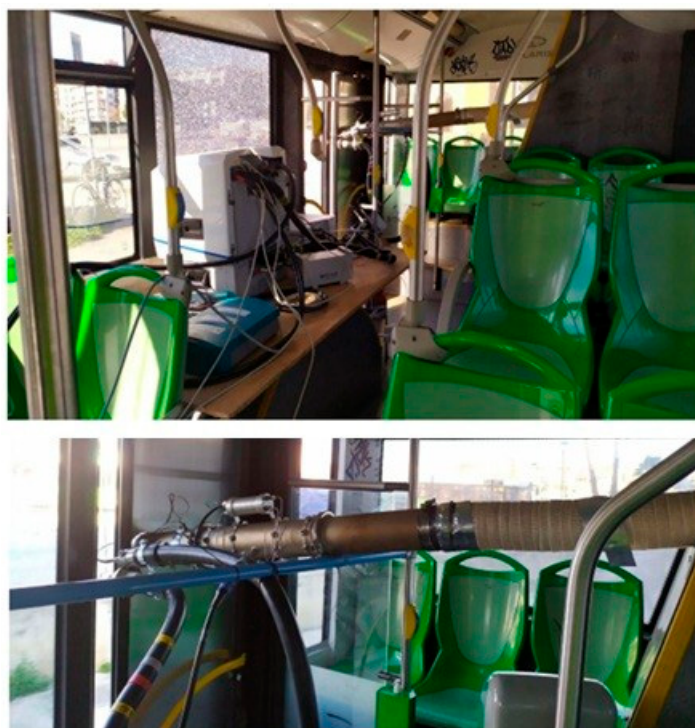
Figure 2. Real photos taken on the bus that show the system used for data acquisition with the components necessary for its operation and the modified exhaust line.
