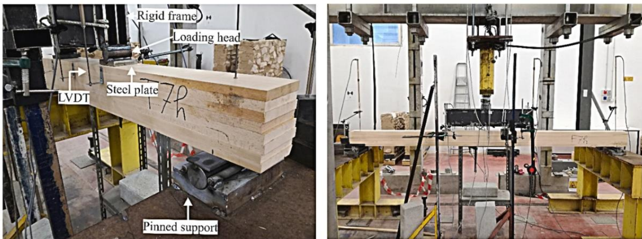
Fig. 3. Set-up left) Equipment details; right) Front view.
