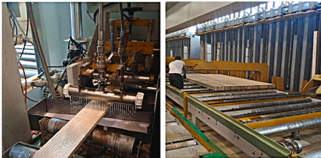
Fig. 1. Glue-laminated timber beams: left) Gluing phase; right) Assembly prior to pressing.
