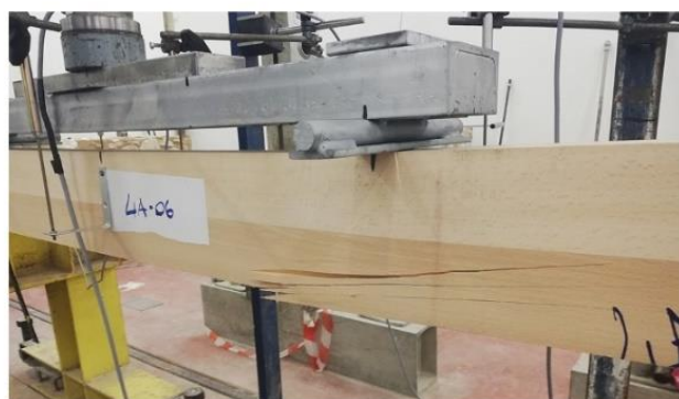
Fig. 7. Typical in-plane bending collapse.
