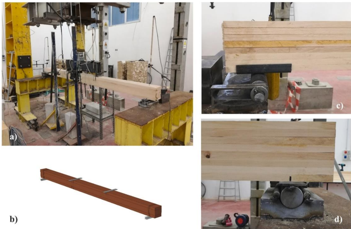
Fig. 11. a) Four-point bending experimental setup, b) FE model beam with ending support and load plates details c) Setup carriage, d) Setup hinge.
