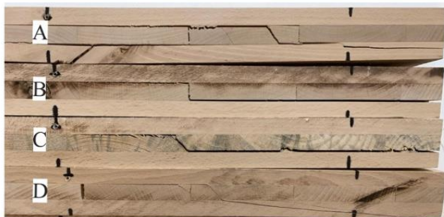
Fig. 5. Collapse patterns of Beech panels in perpendicular-to-plane bending test: A) HB with polyurethane adhesive collapsed for rolling shear and delamination; B) Homogeneous HB panels with polyurethane adhesive collapsed for delamination; C) BP configuration panels collapsed for rolling shear and delamination. D) HB panels with melamine adhesive collapsed for rolling shear.
