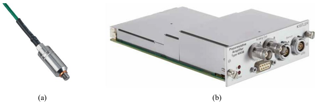
Figure 7-2. Piezoresistive pressure sensor installed on the pump case (a), and Kistler™ signal conditioning system (b).
