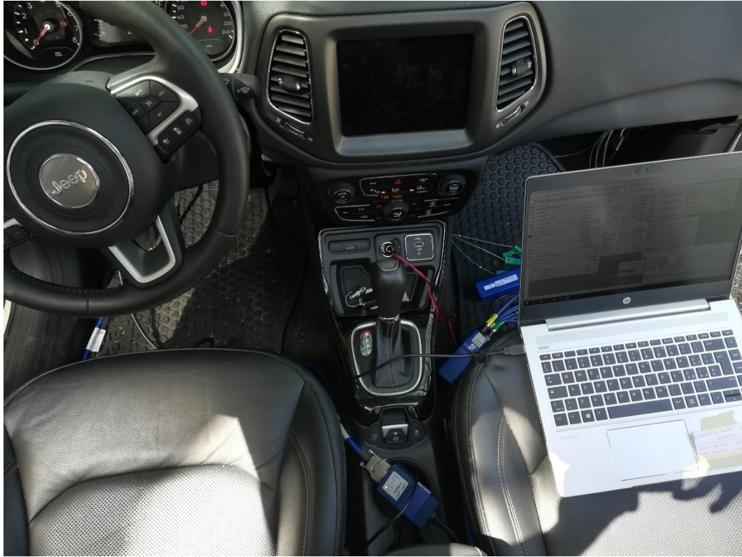
Figure 8-12. Image of the cabin equipped with the INCA-ETAS DAQ system.
