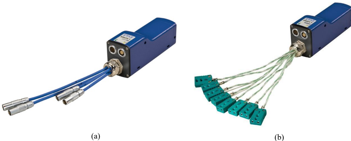
(a) (b) Figure 8-17. ETAS ES413.1 (a) and ES421.1 (b) modules [273,274].
