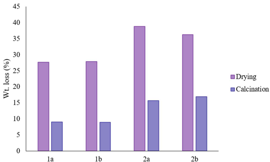
Figure 44. Weight losses of the drying process (105°C, 24 h) and calcination (600°C, 1 h).
