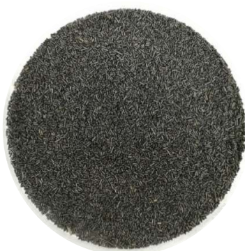
Figure 62. Photographic aspect of the catalyst washed and dried in air for 24 h.
