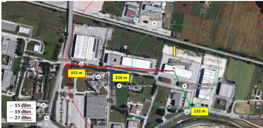
Figure 2.10: Radio coverage tests in case of indoor-outdoor communication (IN-OUT1)
