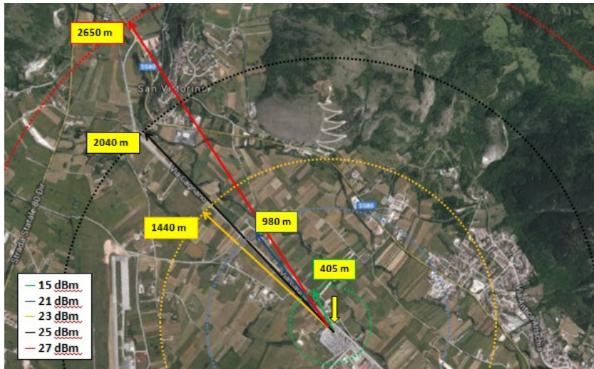
Figure 2.12: Radio coverage tests in case of outdoor communication
