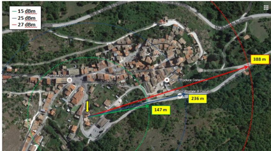
Figure 2.11: Radio coverage tests in case of indoor-outdoor communication (IN-OUT2)
