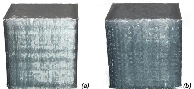
Figure 2. Comparison between two cubes based on the same nominal geometry and manufactured using a different acceleration value.
