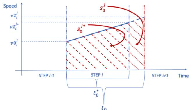
Figure 9. Insufficient distance for acceleration; new end speed.
