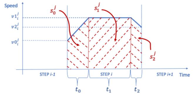
Figure 8. Nominal speed reached during step  $i$ -th.
