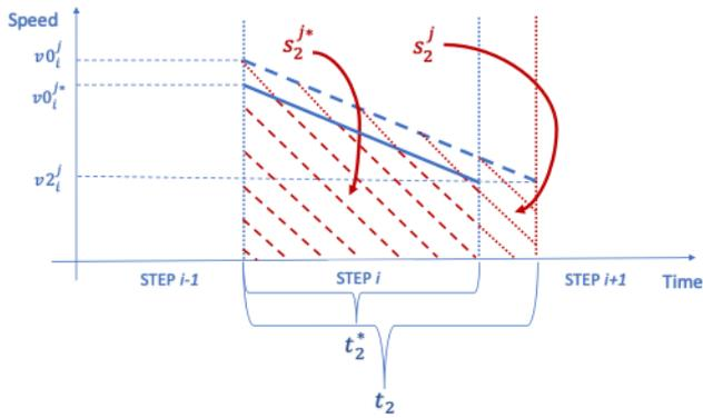
Figure 10. Insufficient space for deceleration; new start speed.
