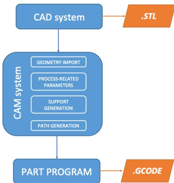
Figure 3. Automatic programming for generating the part program.
