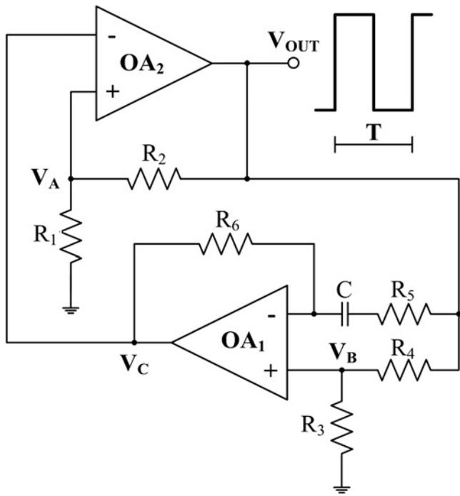
**Fig. 1** Block scheme of the proposed capacitive ( $C$ )/resistive ( $R_5$  or  $R_6$ ) sensor interface
