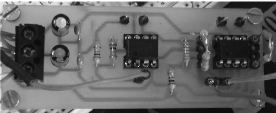
**Fig. 3** Photograph of the fabricated prototype PCB with commercial discrete components
