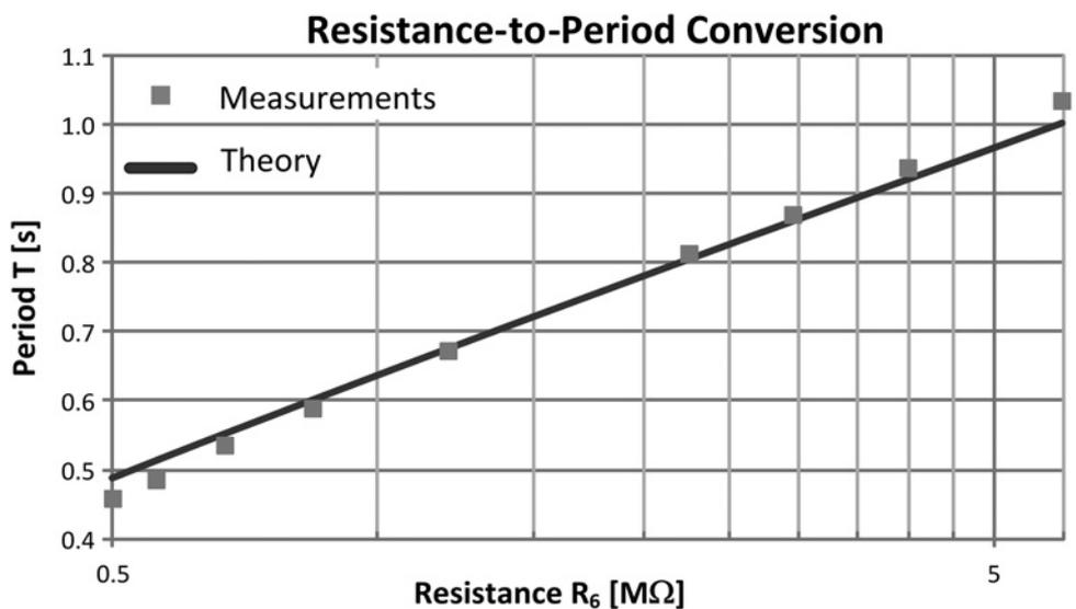
Fig. 6 Theoretical responses and measurement results related to the period  $T$  of the output square waveform against sample resistance  $R_6$
