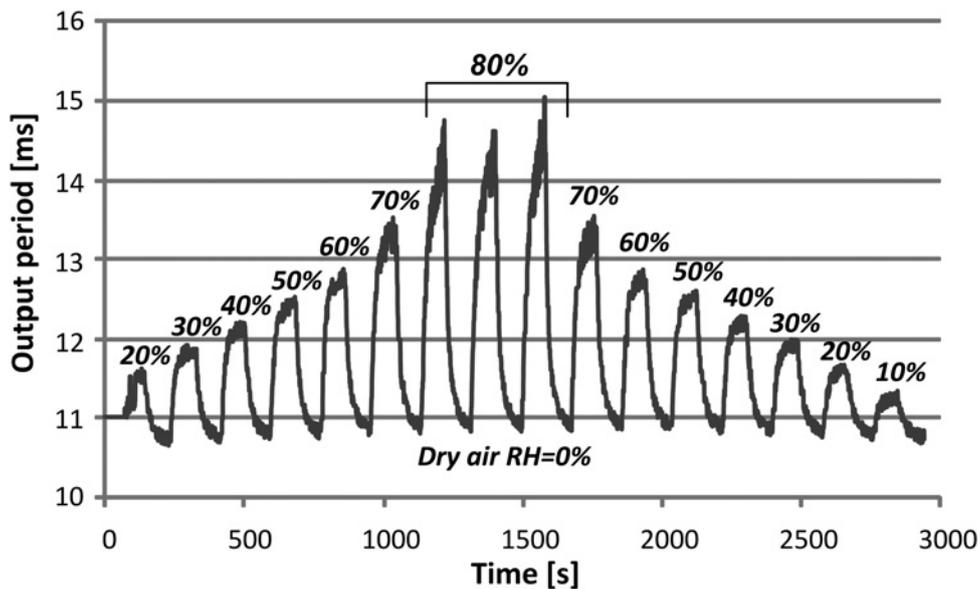
Fig. 7 Experimental measurement showing the output period  $T$  against RH%; the circuit employs a commercial capacitive humidity sensor and OPA350 as OA single supplied at +5 V (i.e. C–T conversion)
