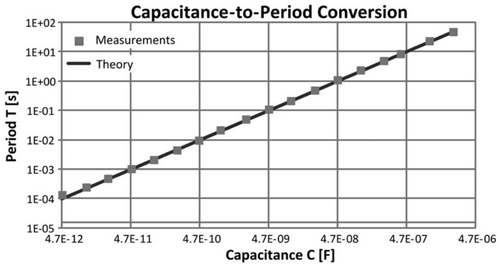
Fig. 4 Theoretical responses and measurement results related to the period  $T$  of the output square waveform against sample capacitance  $C$
