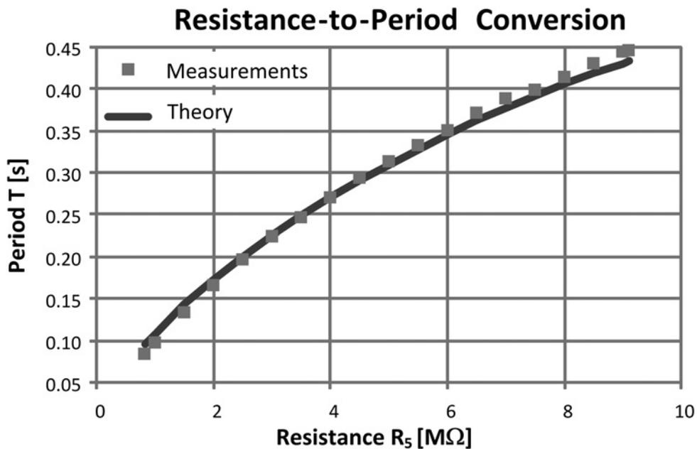
Fig. 5 Theoretical responses and measurement results related to the period  $T$  of the output square waveform against sample resistance  $R_5$
